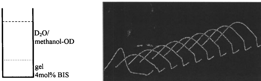
Fig. 10: one-dimensional diffusion experiment (60vol% methanol): left: experimental setup. right: MRI of ten equidistant time-steps (5min \rightarrow 2600min, z-gradient only). The left side of each scan is the top volume (solution) of the experimental setup
